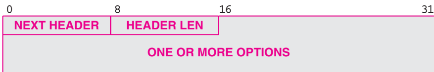
Figure 24.5 Illustration of the IPv6 options extension header with an explicit length.
