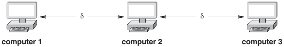
Figure 14.6 Three computers with wireless LAN hardware at maximal distance.
