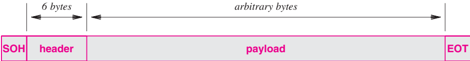
Figure 13.11 An example frame format that uses SOH and EOT characters to delineate a frame.
