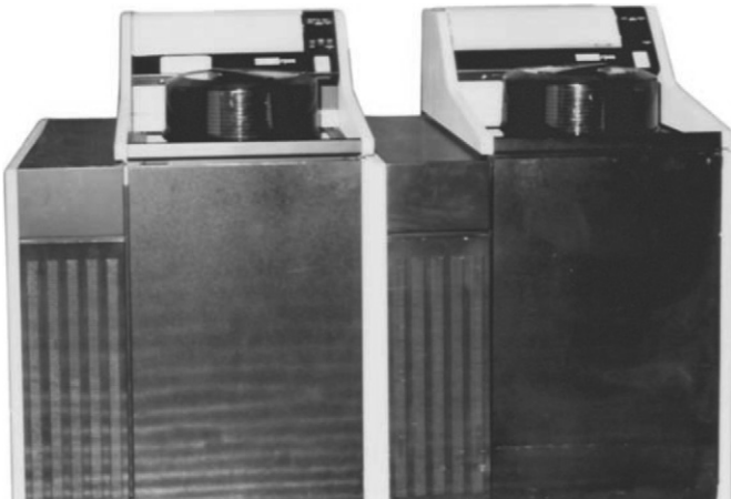
FIGURE e5.17.7 This is a DEC disk drive and the removable pack. These disks became popular starting in the mid-1960s and dominated disk technology until Winchester drives in the late 1970s. This drive was made in the mid-1970s; each disk pack in this drive could hold 80 MB.
