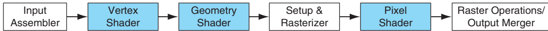
FIGURE B.2.3 Graphics logical pipeline. Programmable graphics shader stages are blue, and fixed-function blocks are white.
