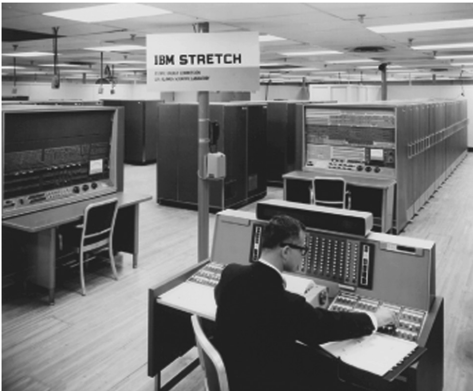
FIGURE e4.16.1 The Stretch computer, one of the first pipelined computers.
