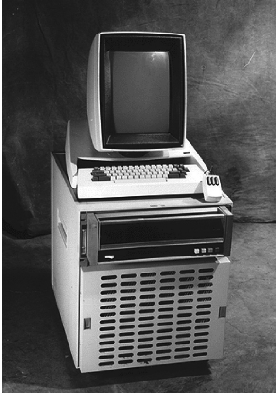
FIGURE e1.12.6 The Xerox Alto was the primary inspiration for the modern desktop computer. It included a mouse, a bit-mapped scheme, a Windows-based user interface, and a local network connection.
