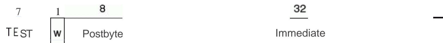
FIGURE 2.45 Typical IA-32 instruction formats. Figure 2.46 shows the encoding of the postbyte. Many instructions contain the I-bit field w , which says whether the operation is a byte or double word. The d field in MOV is used in instructions that may move to or from memory and shows the direction of the move. The ADD instruction requires 32 bits for the immediate field because in 32-bit mode the immediates are either 8 bits or 32 bits. The immediate field in the TEST is 32 bits long because there is no 8-bit immediate for test in 32-bit mode. Overall, instructions may vary from 1 to 17 bytes in length. The long length comes from extra 1-byte prefixes, having both a 4-byte immediate and a 4-byte displacement address, using an opcode of 2 bytes, and using the scaled index mode specifier, which adds another byte.
