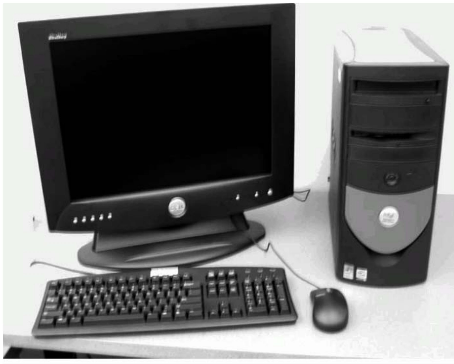
FIGURE 1.6 A desktop computer. The liquid crystal display (LCD) screen is the primary output device, and the keyboard and mouse are the primary input devices. The box contains the processor as well as additional I/O devices. This system is a Dell Optiplex GX260.
