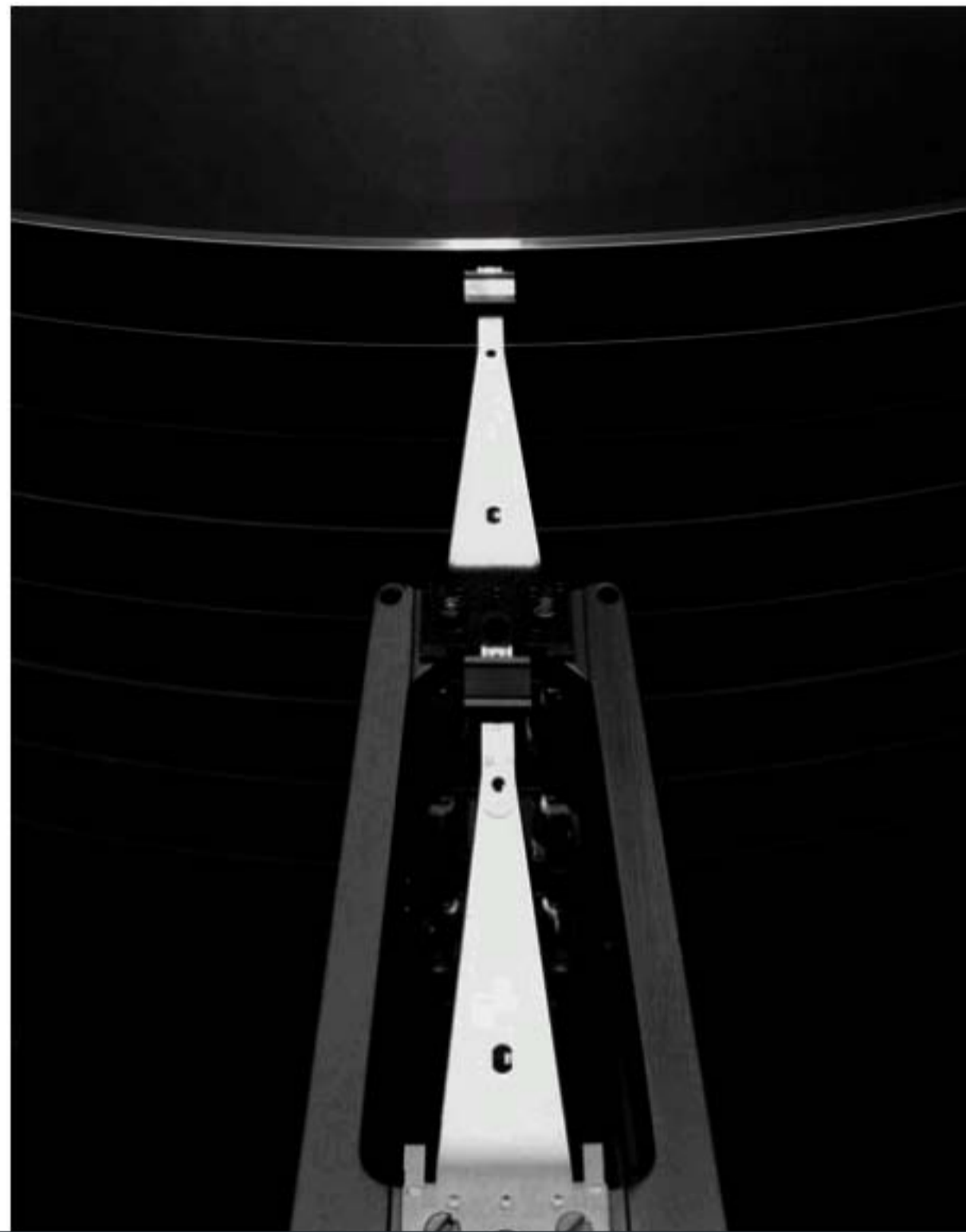
FIGURE 1.11 A disk showing 10 disk platters and the read/ write heads.
