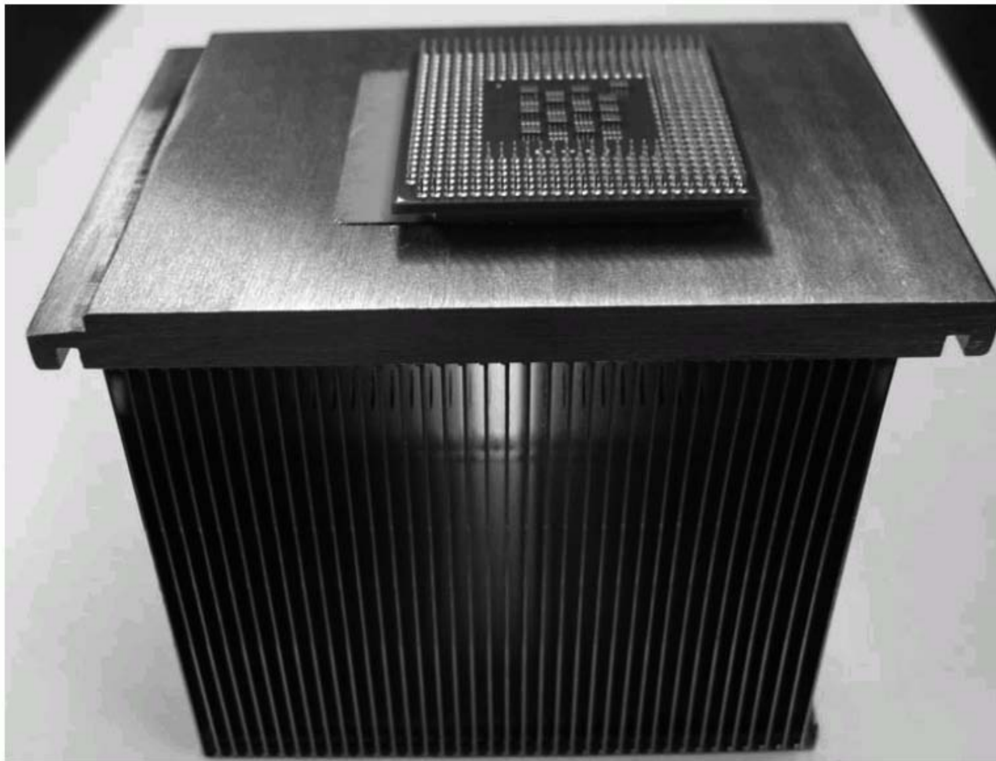
FIGURE 1.16 An Intel Pentium 4 (3.06 GHz) mounted on top of its heat sink, which is designed to remove the 82 watts generated within the die.
