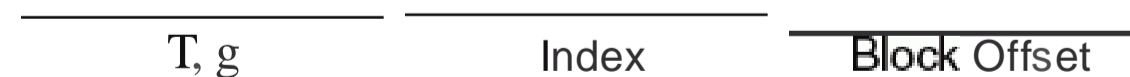
FIGURE 7.16 The three portions of an address in a set-associative or direct-mapped cache. The index is used to select the set , then the tag is used to choose the block by comparison with the blocks in the selected set. The block offset is the address of the desired data within the block.
