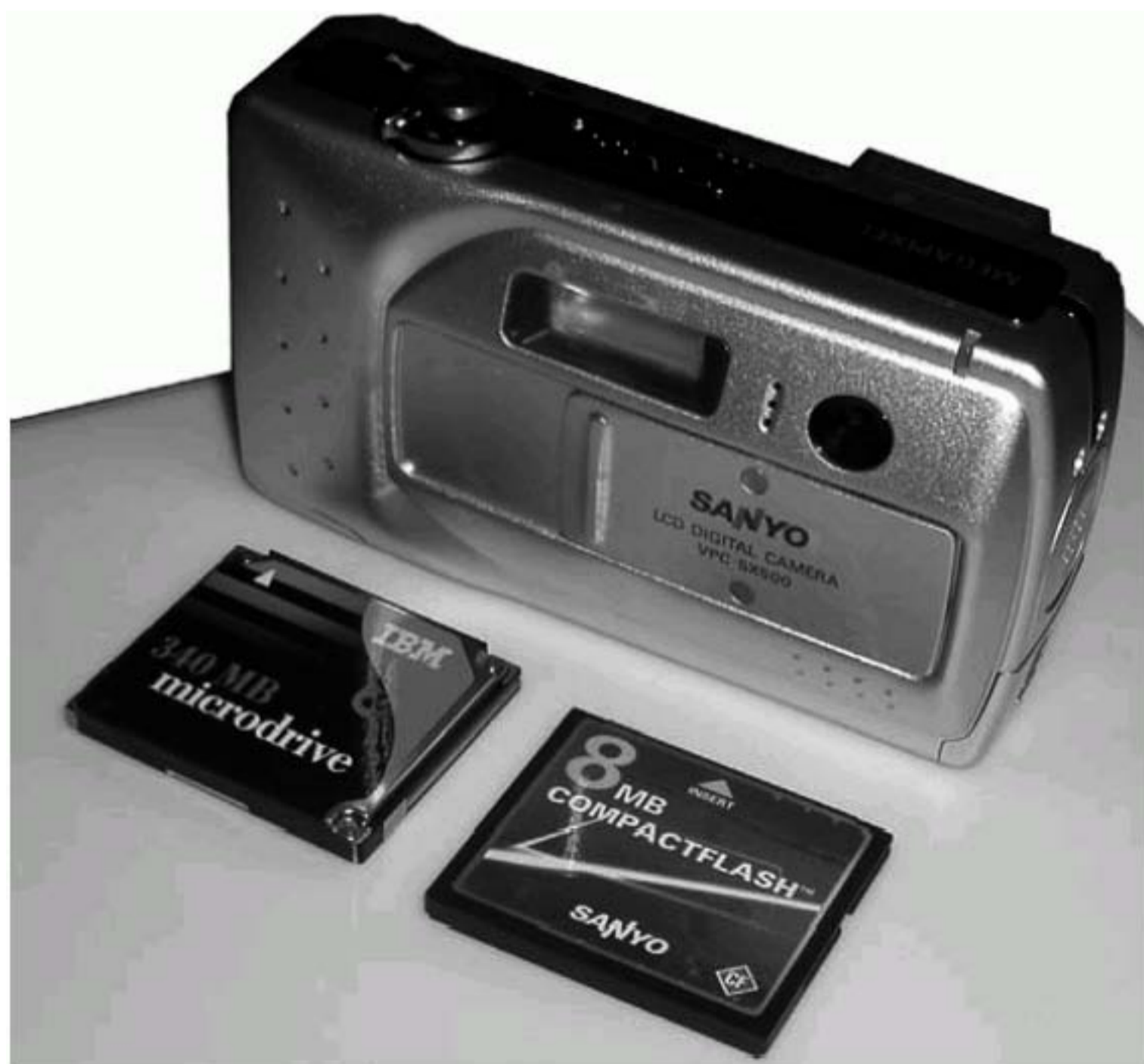
FIGURE 8.14 The Sanyo VPC-SXS00 with Flash memory card and IBM Microdrive. Although newer cameras offer more pixels per picture, the principles are the same. This 1360 x 1024 pixel digital camera stores pictures either using CompactFlash memory or using a IBM Microdrive. This photo was taken using a 340 MB microdrive and a 8 MB CompactFlash memory. As Figure 8.15 shows, in 2004 the capacities are as large as 1 GB to 4 GB it is 4.3 inches wide x 2.5 inches high x 1.6 inches deep, and it weighs 7.4 ounces. In addition to taking a still picture and converting it to JPEG format every 0.9 seconds, it can record a Quick Time video clip at VGA size (640 x 480). One technological advantage is the use of a custom system on a chip to reduce size and power, so the camera only needs two AA batteries to operate versus four in other digital cameras.
