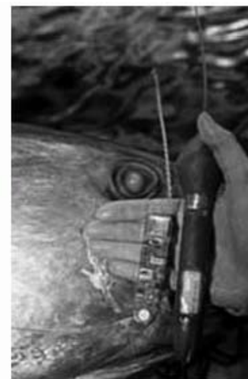
A pop-up archival satellite tag and internal electronics.
